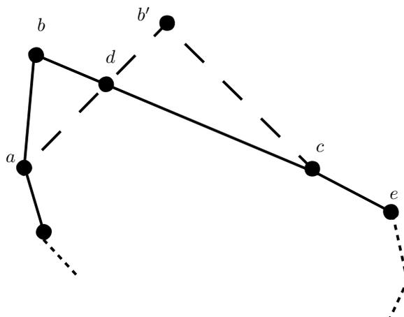
FIG. 10: Changing edge lengths can change convexity.
